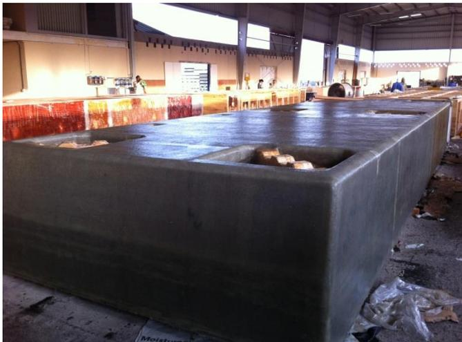
Photos of the production of FRP pontoons starting with the timber frame and then entirely encapsulated in fibre reinforced polymers to provide an extremely strong floating pontoon
